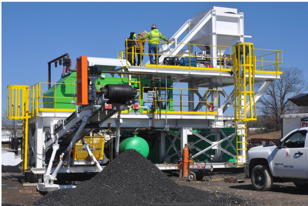
Figure 11. Photograph of a recent production-scale installation of the DriJet™ sorter technology.
